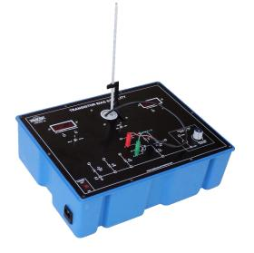
**OMEGA TYPE ETB-60** Experimental Training Board has been designed specifically to study the Transistor Bias Stability.
