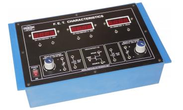
**OMEGATYPE ETB-53** Experimental Training Board has been designed specifically to study the characteristics of a Field Effect Transistor. The board is absolutely self contained and requires no other apparatus.
