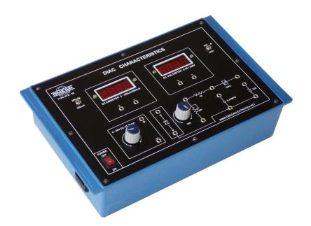
**OMEGA TYPE ETB-66** Experimental Training Board has been designed specifically to study the characteristics and applications of a DIAC. DIAC is extensively used now a days in power control circuits.
