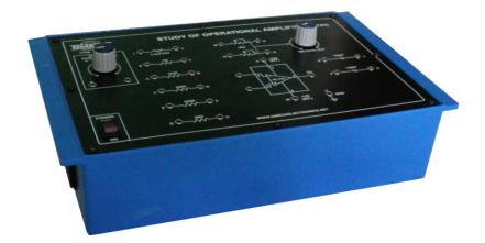
**OMEGA TYPE ETB-71** Experimental Training Board has been designed specifically for the study of Operational Amplifier (mA741).
