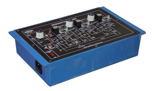
OMEGA TYPE ETB-63 Experimental Training Board has been designed specifically to study the working and construction of Sequential Timer. It consists of three timers connected in cascade to form a sequential timer. The time period of each timer can be set independently. Timers are very useful in industrial applications such as automatic control, automatic testing, sequential operations of machines etc. The board is absolutely self contained and requires no other apparatus.
