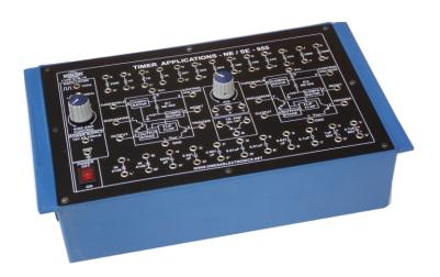
**OMEGA TYPE ETB-76** Experimental Training Board has been designed specifically to study various applications of Timer IC 555. This Training Board is useful to realise 50% Duty Cycle Oscillator, Ramp Generator, Time Delay Circuit, Sequence Generator, Schmitt Trigger, Monostable Multivibrator, Astable Multivibrator, Pulse Width Modulator, Pulse Position Modulator etc.
