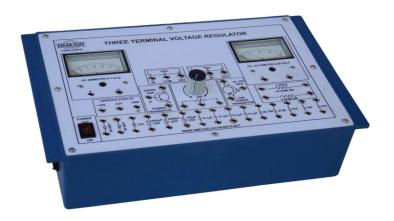
OMEGA TYPE ETB-87 Experimental Training Board has been designed specifically for thorough understanding of Three Terminal Voltage Regulators of 78XX and 79XX series. Although these two series of regulators are designed for fixed voltage regulation, this training board explores various methods of raising the output voltage and also to continuously vary their output voltage.
