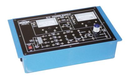
**OMEGA TYPE ETB-88** Experimental Training Board has been designed specifically for the study of D.C. Power Supplies using basic techniques of rectification, smoothing and regulation.
