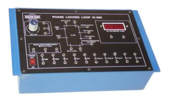
**OMEGA TYPE ETB-90** Experimental Training Board has been designed specifically for the study of Phase Locked Loop (PLL) IC 565. This training board covers most of the important parameters, characteristics and applications on Phase-locked Loop (PLL) IC 565.
