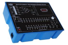
**OMEGA TYPE ETB-93** Experimental Training Board has been designed specifically to study the behavior of the Reactive Elements and Time Dependent Network Analysis.
