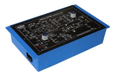
**OMEGA TYPE ETB-94** Experimental Training Board has been designed specifically on sinusoidal Oscillators. In this training board all the basic sinusoidal oscillator circuits can be quickly and easily assembled and studied.
