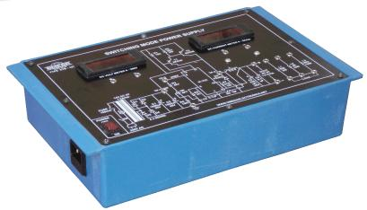
**OMEGA TYPE ETB-107** Experimental Training Board has been designed to practically demonstrate the operation of a Switching Mode Power Supply. The Switching waveform and various voltages can be observed on the test points provided on the panel.
