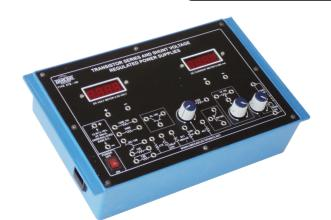
OMEGA TYPE ETB-108 Experimental Training Board has been designed specifically for the study of transistorised series and shunt voltage regulated power supplies. Apart from series and shunt circuits, the current limiting and variable voltage techniques are also included. The board is absolutely self contained and requires no other apparatus.
