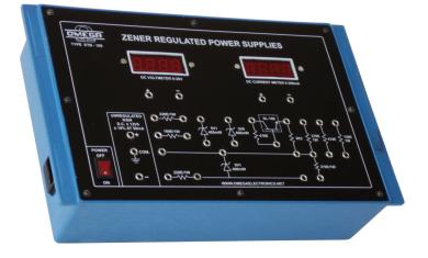
**OMEGA TYPE ETB-109** Experimental Training Board has been designed specifically for the study of regulated power supplies based on Zener Voltage regulating diodes. A Zener diode is generally employed in a standard circuit as a voltage regulator. This training board deals with some more possible voltage regulating circuits apart from the standard one. The board is absolutely self contained and requires no other apparatus.
