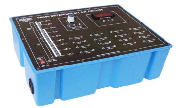
**OMEGA TYPE ETB-103** Experimental Training Board has been designed specifically for the complete study of the phase difference in L.C.R. circuits. A selection of L,C and R values have been provided and phase difference in various combinations of L-C, L-R, C-R and L-C-R circuits can be studied in depth. The board is absolutely self contained and requires no other apparatus.
