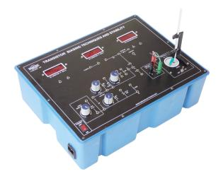
**OMEGA TYPE ETB-105** Experimental Training Board has been designed specifically to study different biasing techniques for transistor amplifier circuits. Also the effect of transistor replacement (change in b) and temperature changes can be studied on all biasing circuits.
