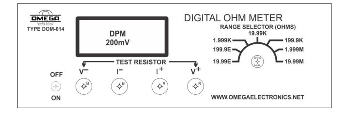
OMEGA TYPE DOM-14 is suitable for measurement of resistance of various kinds of resistors and resistive components and is useful for incoming inspection departments and production line testing of resistors. The usage of latest MOS LSI technology has helped in increasing the reliability, ease of servicing and making the instrument light weight and compact.
