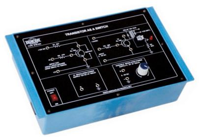
**OMEGA TYPE ETB-223** has been designed specifically to study switching characteristics of a transistor and its application.
