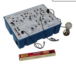
OMEGA TYPE ETB-224 Experimental Training Board has been designed specifically to study application of Thermistors Type PTC & NTC).
