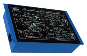
OMEGA TYPE ETB-225 has been designed specifically for study current series, current shunt, voltage series and voltage shunt Feed Back Amplifier using Transistors.
