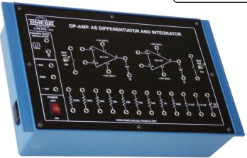
**OMEGA TYPE ETB-216** Experimental Training Board has been designed specifically for the study of OP-AMP IC's applications. This training board covers Integrator and Differentiation application of operational amplifiers (IC-741) and makes the student familiar with it.
