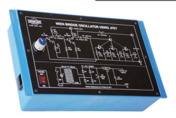
OMEGA TYPE ETB-227 The experimental set up has been designed specially for the study of Wien Bridge Audio Oscillator using JFET. The Training board helps us to under stand the utilization of Audio OSC and obtain oscillation at different frequencies.
