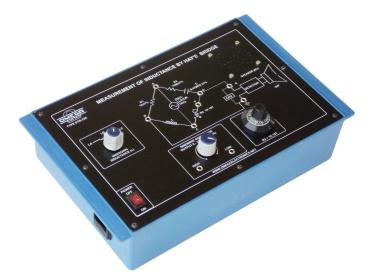
**OMEGA TYPE ETB-228** Experimental Training Board has been designed specifically to measure the value of unknown inductance by Hay's bridge.
