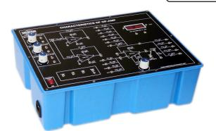
**OMEGA TYPE ETB-242** Experimental Training Board has been designed specifically for the study of OP-AMP CHARACTERISTICS ICs 741.
