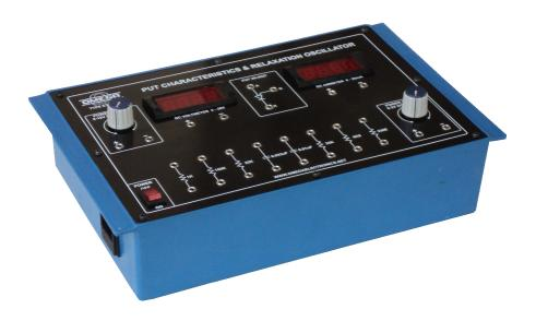
**OMEGA TYPE ETB-243** Experimental Training Board has been designed specifically for the study of PUT characteristics & its relaxation oscillator.
