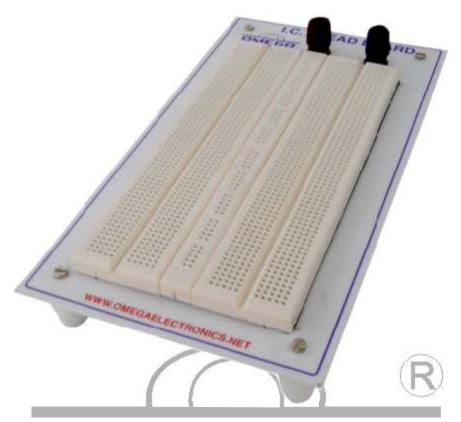
**OMEGA TYPE BBS-101, BBS-102, BBS-103** I.C. Bread Board Systems have been designed to provide instant circuit construction without soldering on the bread board area .Learners can insert components directly on breadboard and make all interconnections as required with 24 Swg (Gauge) solid wire. Within few minutes they can complete their projects/design on the same.
