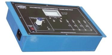
**OMEGA TYPE ETB-240** Experimental Training Board has been designed specifically for the study of Voltmeter Characterstics : Ohms per volt. It is actual practice to specify the sensitivity of a voltmeter in terms of ohms per volt.
