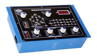
OMEGA TYPE ETB-241 Experimental Training Board has been designed specifically for the study of Wheatstone Bridge. Using this bridge the value of unknown resistor can be found. The board is absolutely self contained and requires no other apparatus.
