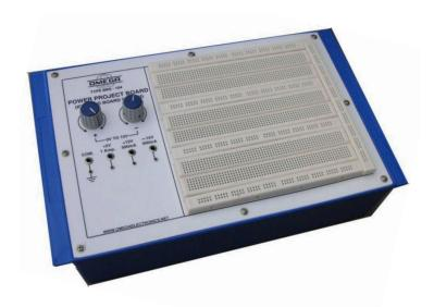
**OMEGA TYPE BBS-104** Power Project Board System has been designed to provide instant circuit construction without soldering on the bread board area. Learners can insert components directly on breadboard and make all interconnections as required with 24 Swg (Gauge) solid wire. Within few minutes they can complete their projects/design on the same.
