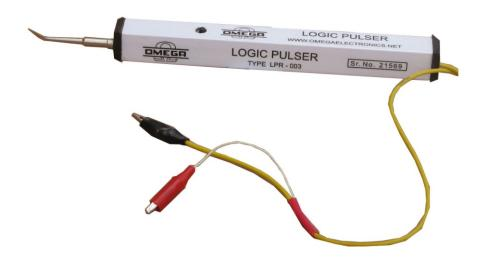
**OMEGATYPE LPR-003** Logic Pulser is a single short duration pulse generator packed in a convenient, easy to use probe body. Its function is to over-ride the naturally occurring state at the particular circuit node under test. That is, pulse selection is automatic and the high output current capability (source or sink) allow it to over-ride high & low states.
