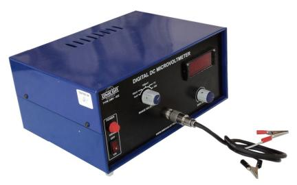
**OMEGA TYPE DMV-022** Digital D.C. Micro voltmeter is very versatile multipurpose instrument for the measurement of low dc voltage. It has 5 decade ranges from 1mV to 10V with 100% over-ranging. For better accuracy and convenience, readings are directly obtained on 3½ digit LED display. IC amplifier used offers exceptionally low offset voltage and input bias parameters, combined with excellent speed characteristics.
