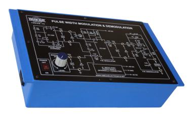
**OMEGA TYPE ETB-113** Experimental Training Board has been designed to study on the modern techniques of Pulse Width Modulation / Demodulation. Using this training board one can know the specialized techniques of Pulse Width Modulation and Demodulation.
