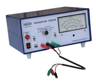
**OMEGA TYPE TT-285** Transistor Tester is a simple appratus for carrying out quick checks on PNP and NPN transistors. Due to its simple design and small dimensions, the tester is specially suitable for repair shops and service purpose. In addition, it enables semi-conductor diodes to be checked for quiescent current. The transistor tester is housed in a metal cabinet with enamel finish and processed siliver grey front panel.
