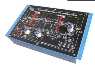
OMEGA TYPE ETB-212 Experimental Training Board has been designed specifically to study Pulse Code Modulation & Demodulation. In the basic PCM Modulator the base band analog signal is covered into 8 bit digital format using an ADC. The sampling rate is set at 2.5 KHz. The 8 bit parallel data from ADC is converted into serial bit stream at 33 kbps.
