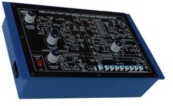
**OMEGA TYPE ETB-208** Experimental Training Board has been designed specifically for the study of Amplitude shift key modulation and demodulation.
