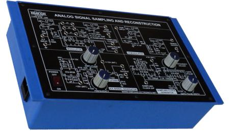
OMEGA TYPE ETB-220 Experimental Training Board has been designed specifically to study of Sampling Theorem using Pulse Amplitude Modulation and Demodulation. The training board is complete in all respect except C.R.O.
