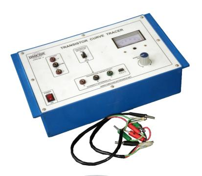
**OMEGA TYPE DB-3** Dynamic Demonstration Board has been specifically designed to display the transfer characteristics of NPN/PNP transistor on a C.R.O. The board has an excellent educational use as it permits the students to see the transistor in action.
