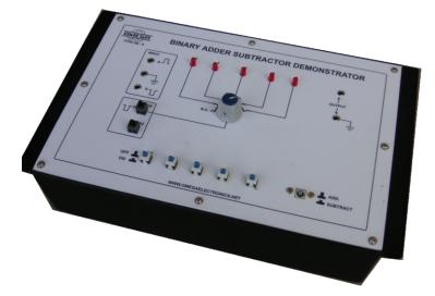
OMEGA TYPE DB-4 Demonstration Board has been designed specifically to understand the methods of addition, subtraction and multiplication in binary system. Digital Systems are based on Binary System of counting therefore it becomes essential to master this system. The board is absolutely self contained and requires no other apparatus.
