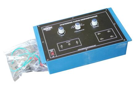
OMEGA TYPE DB-2 Dynamic Demonstration Board has been designed specifically for the Demonstration of Hysteresis Curve. Without the aid of modern techniques, the display of Hysteresis loop can be a long and tedious demonstration and, in the past, the college laboratories have found it difficult to carry out such an experiment. Now the display of B-H loop has comparatively become a simple matter with OMEGATYPE DB-2 Hysteresis Curve Demonstrator.
