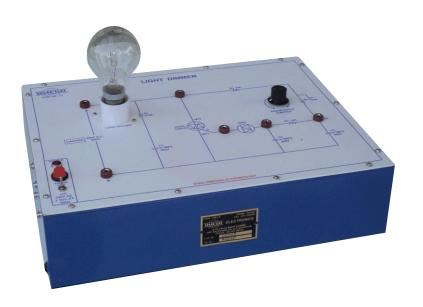
**OMEGA TYPE DB-21** Dynamic Demonstration Board has been designed specifically for the study of Light Dimmer. This Training Board gives a better understanding of the principle of phase control using Diac & Triac.
