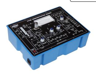
OMEGA TYPE DB-13 Dynamic Demonstration Board has been designed specifically for the demonstration of VTVM circuit based on two vacuum tubes. Complete circuit schematic is drawn on the panel with various controls and sockets at required places. The required circuit for an experiment can be easily assembled with the help of patch cords. The design of this Demonstration Board enables a student to perform experiments to understand the basic concepts as also the working of complete VTVM.
