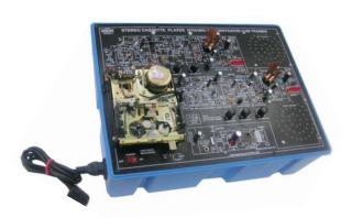
**OMEGA TYPE DB-16** Stereo Cassette Player Dynamic Demonstrator cum Trainer has been designed with a view to provide practical/experimental knowledge of the latest circuit of IC based Stereo Cassette Player on Single glass epoxy PCB, with Fault Creating Facility.
