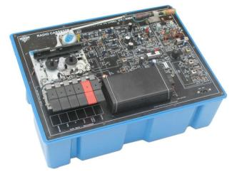
**OMEGA TYPE DB-17** Radio Cassette Recorder (Two-in-one) Dynamic Demonstrator-Cum-Trainer has been designed with a view to provide practical/experimental knowledge of the circuit of IC based Radio Cassette Recorder on Single glass epoxy PCB with fault creating facility.
