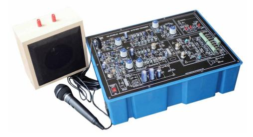
**OMEGA TYPE DB-27** This Trainer has been designed with a view to provide practical and experimental Knowledge of general circuit of PA (Public Address) System Trainer on Single P.C.B. of size  $11\frac{1}{4} \times 15\frac{1}{4}$ ".
