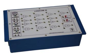
OMEGA TYPE LTB-808 Computer Logic Training Board has been designed specifically for the use of students in digital electronic lab. The students can build-up various logic functions and understand their working i.e. Full Adder, Half Adder, Even Parity Check, Odd Parity Check, Exclusive OR and different type of Logic Circuits. The board is absolutely self contained and requires no other apparatus.
