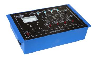
OMEGA TYPE LTB-813 Computer Logic Training Board has been designed specifically for the study of Digital to Analog Conversion and to make the students familiar with the basic principle & techniques of "Digital to Analog Conversion". Input state switches with storage register are provided to feed the derived digital input and analog output can be read directly on a voltmeter in terms of voltage. The board is absolutely self contained and requires no other apparatus.
