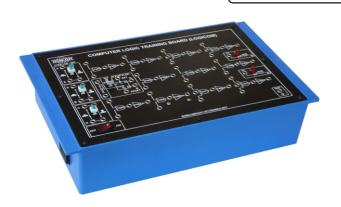
**OMEGA TYPE LTB-805** Computer Logic Training Board has been designed specifically to study the compound logic functions like Full Adder, Half Adder, Even Parity Check, Odd Parity Check, Exclusive OR and different types of Filp-Flops. These all can be synthesized from the most fundamental logic function NAND. The board is absolutely self contained and requires no other apparatus.
