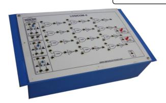
OMEGA TYPE LTB-807 Computer Logic Training Board has been designed specifically for the use of students in digital electronic lab. The students can build-up various logic functions and understand their working i.e. Full Adder, Half Adder, Even Parity Check, Odd Parity Check, Exclusive OR and different type of Logic Circuits. The board is absolutely self contained and requires no other apparatus.
