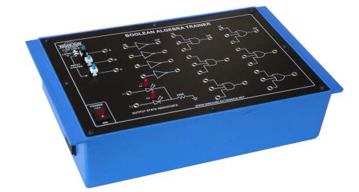
**OMEGA TYPE LTB-818** Computer Logic Training Board has been designed specifically on Boolean Algebra to study the Boolean Algebraic theorems and verification of the same. By using the clearly marked built-in logic gates, students can implement logic circuits for verification of Boolean Algebraic theorems. The board is absolutely self contained and requires no other apparatus.
