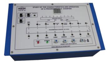
**OMEGA TYPE LTB-821** Computer Logic Training Board has been designed specifically for the study & Operation of Programmable Counter to give students an idea about Programmable Counters and different modes of the same. The output of counter can be observed in decimal code with the help of seven segment displays. The board is absolutely self contained and requires no other apparatus.
